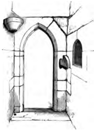
Doorway into Cloisters, shewing the Stone Socket for Pivot and Stone Catch for the Latch, Franciscan Abbey.
